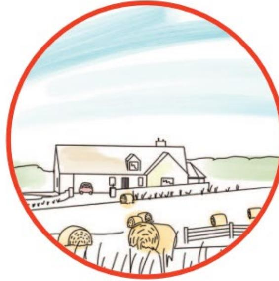
Drawing illustrates unacceptable siting, the proposal lacks immediately adjoining landform, mature trees, established woodland or buildings of a sufficient scale to provide acceptable enclosure, containment and backdrop.
